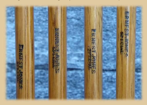
The shafts have received 30 layers of natural shellac using the old French Polish technic.
